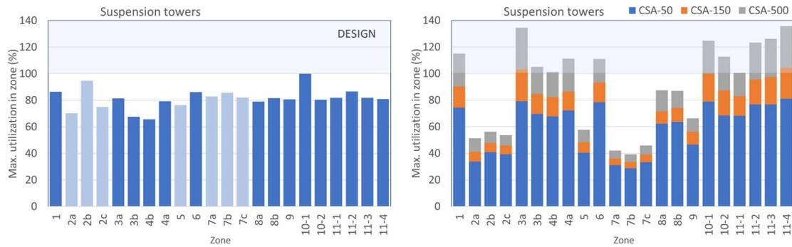
**FIGURE 23** Highest utilization in all suspension towers by zone. Results for DESIGN loading<sup>21</sup> is to the left and CSA loading to the right. Includes all load cases described in chapter 3.3.
