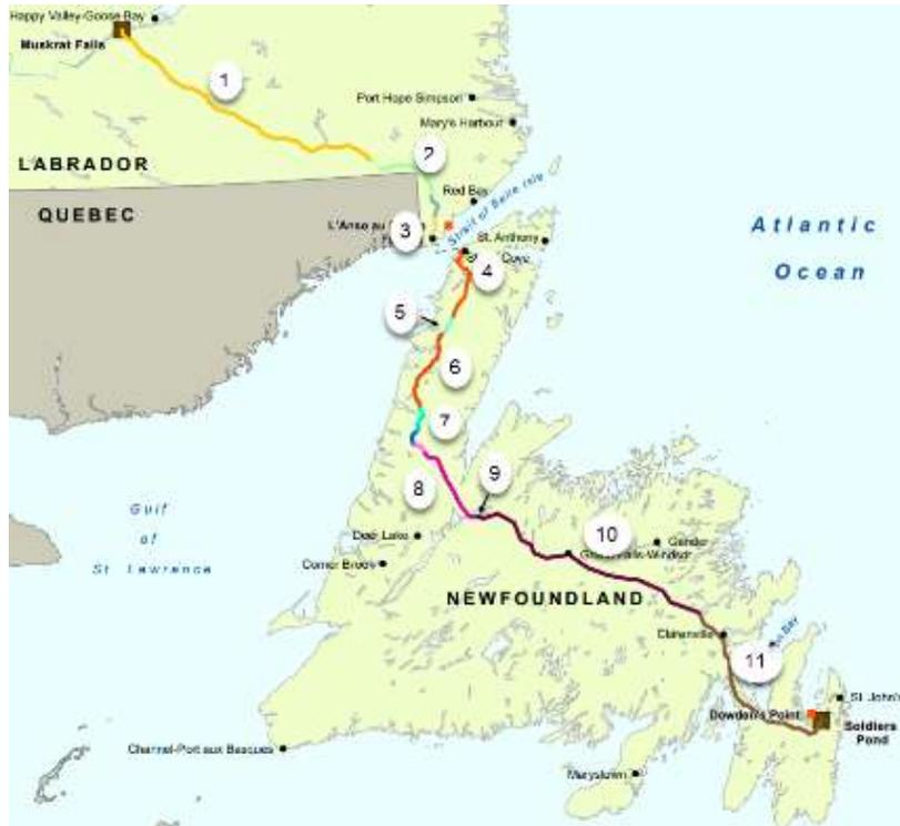
FIGURE 2 LITL Transmission Route and Meteorological Zones.
