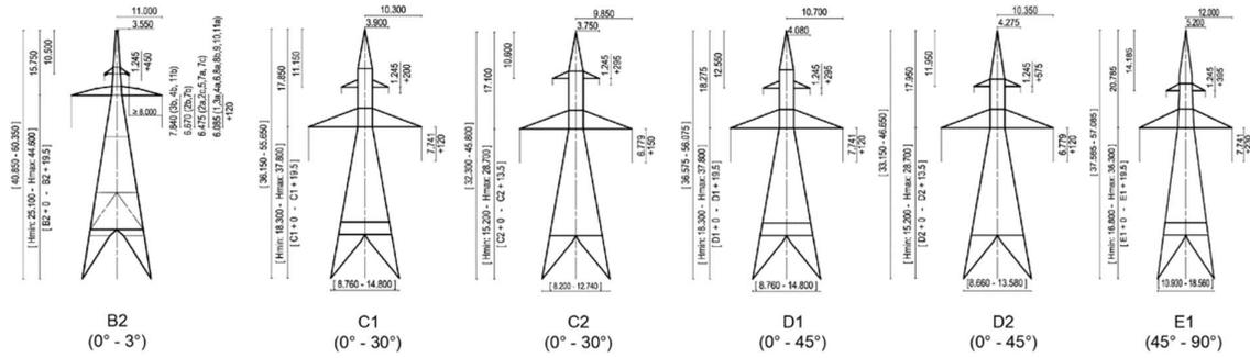
**FIGURE 4** Tower geometries for self-supporting towers.
