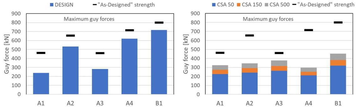
**FIGURE 29** Maximum guy forces for each tower type in the analysis. The “As-Designed” values used in the design of all guys are shown with a black line and compared to DESIGN loading on the left figure and to the CSA loading on the right figure.
