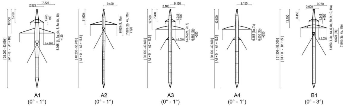
**FIGURE 3** Tower geometries for guyed towers.
