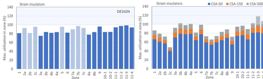
**FIGURE 34** Tension insulators, highest utilization in each loading zone. Utilization in DESIGN loading<sup>21</sup> is to the left and CSA loading to the right.
