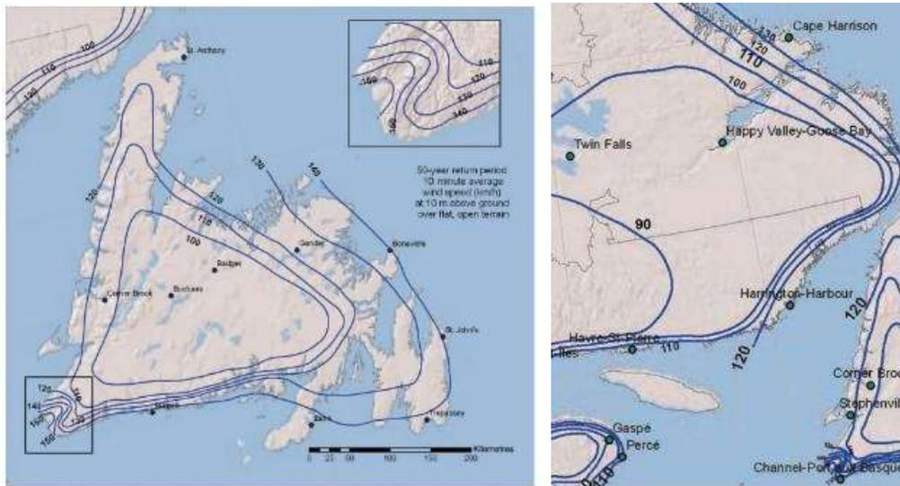
**FIGURE 17** Reference 50-year return period wind speed (km/h) for Newfoundland and Labrador, Figures CA.1 and CA.3 in the CSA standard.
