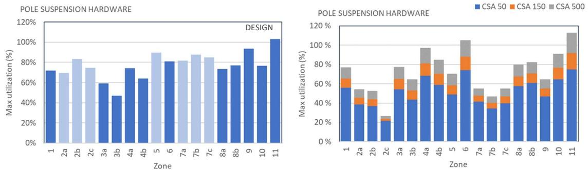
FIGURE 36 Pole conductor suspension hardware. Maximum utilization per zone of DESIGN<sup>21</sup> loading (left) and CSA- loads (right) is presented.
