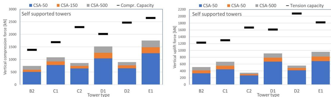
**FIGURE 28** Maximum axial force on tower foundation in self-supporting towers<sup>24</sup> and comparison to force used in the design of foundations. The vertical compression force is to the left and vertical uplift force to the right.
