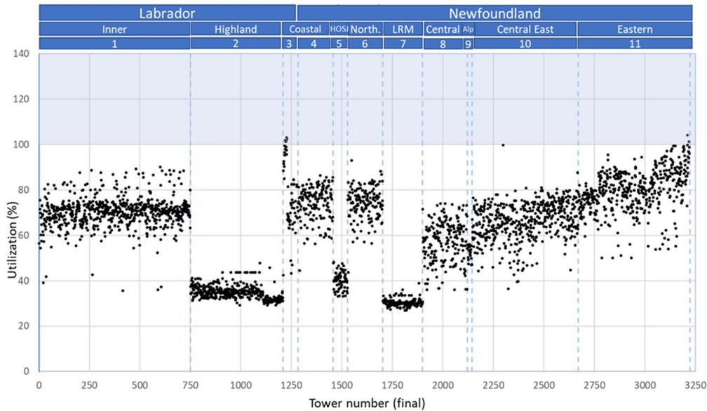
FIGURE 25 CSA-150 loading, highest utilization in all suspension towers. Includes all load cases described in chapter 3.2.
