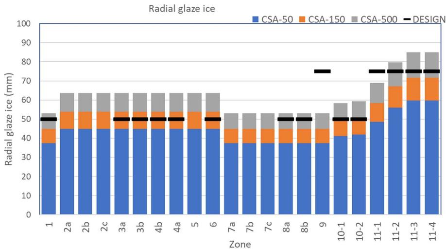
**FIGURE 20** Radial glaze ice loading, CSA-50, CSA-150, CSA-500 and DESIGN.
