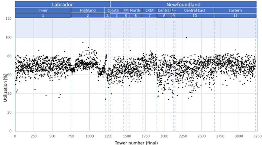
FIGURE 22 Utilization in all suspension towers for DESIGN loading.
