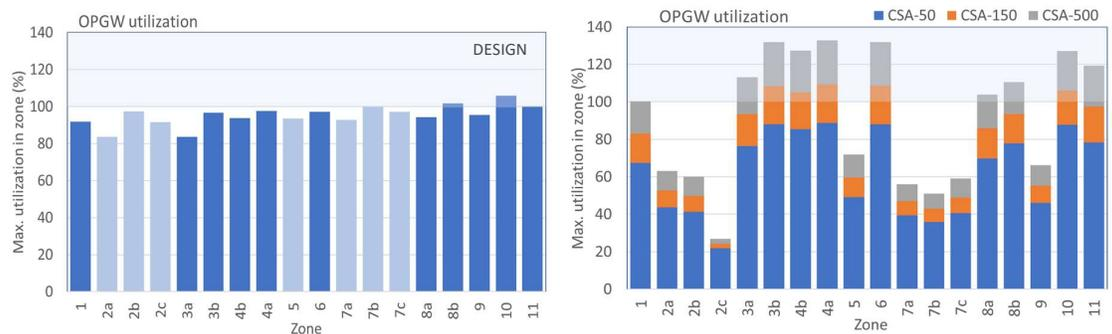
**FIGURE 32** OPGW Conductor, highest utilization in each loading zone. Utilization in DESIGN loading<sup>21</sup> is shown to the left and CSA loading to the right.
