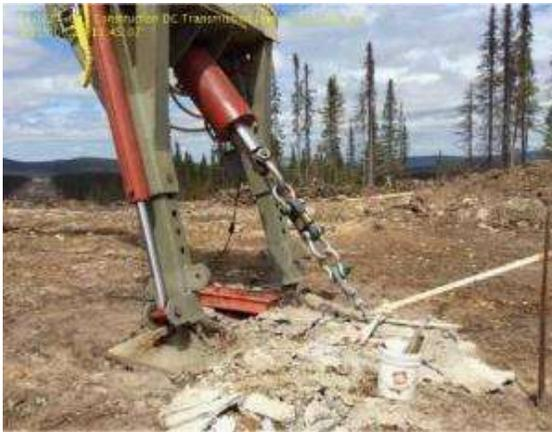
**FIGURE 13** Guy anchor testing.
