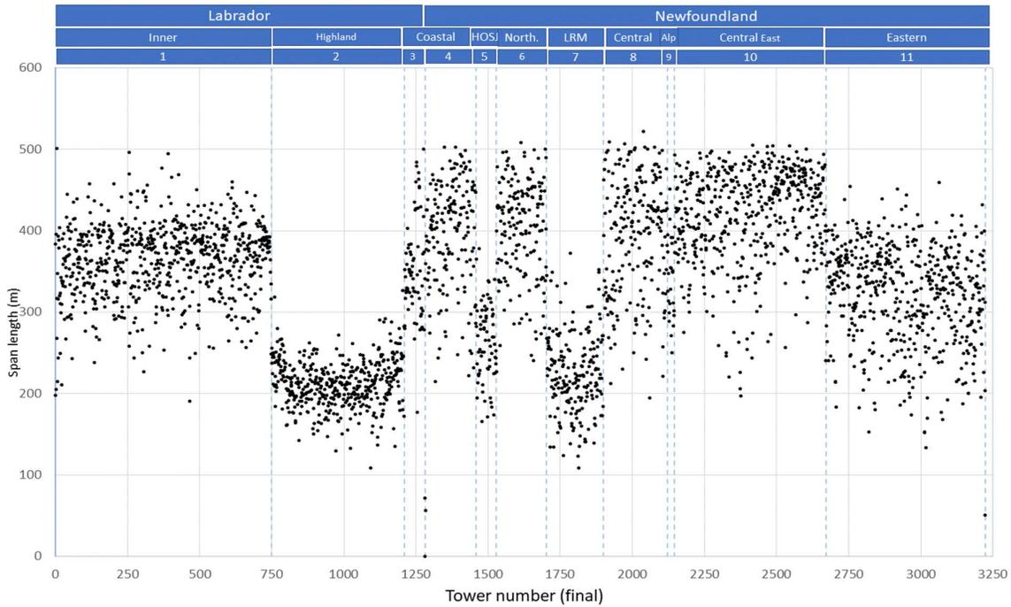
**FIGURE 10** Span lengths (m) along the line route of LITL.
