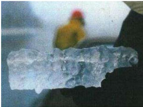
**FIGURE 15** Glaze ice from the conductor, 1984 storm. Photo from ref. [11].
