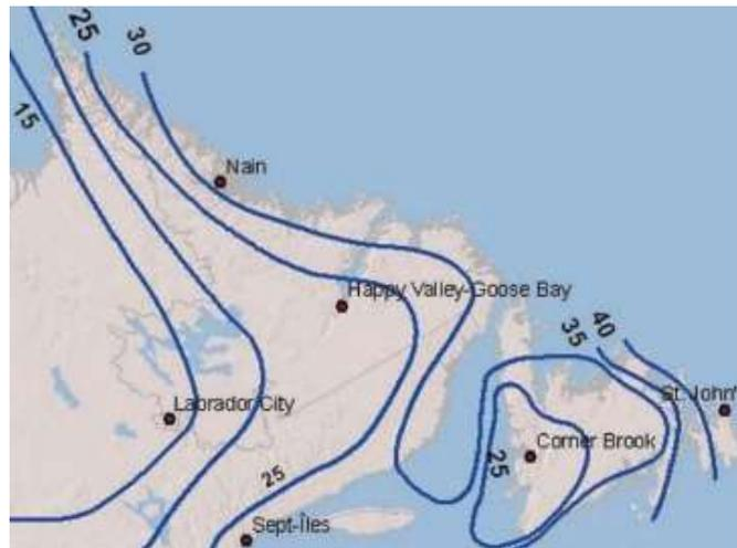
**FIGURE 19** Reference 50-year return period of glaze ice thickness(mm) from freezing precipitation for Newfoundland and Labrador, figures CA.10 in the CSA standard. The structural load is obtained by adding spatial factor and height factor to these values.
