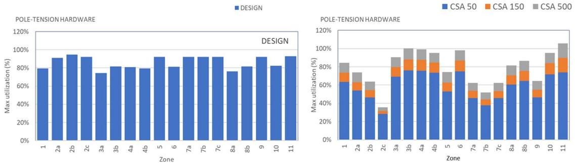
FIGURE 35 Pole conductor tension hardware. Maximum utilization per zone of DESIGN<sup>21</sup> loading (left) and CSA- loads (right) is presented.
