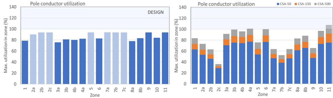
**FIGURE 30** Pole Conductor, highest utilization in each loading zone. Utilization in DESIGN loading<sup>21</sup> is to the left and CSA loading to the right.
