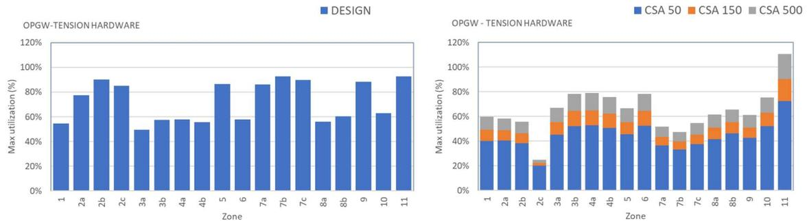
FIGURE 39 OPGW tension hardware. Maximum utilization per zone of DESIGN<sup>21</sup> and CSA- loads is presented.
