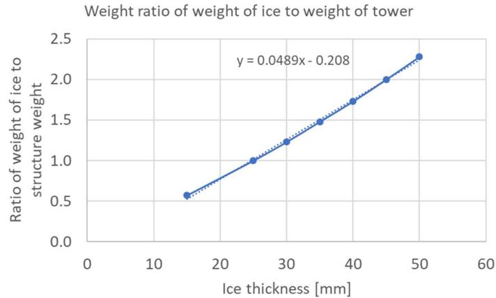
**FIGURE 21** CSA alternative approximation of ice weight on tower based on tower weight and ice thickness.
