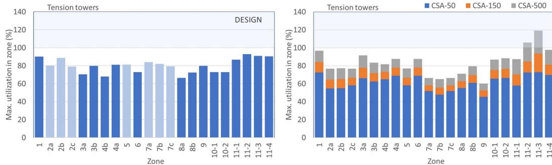
**FIGURE 26** Highest utilization in tension towers<sup>21</sup> in the load cases “Max. Ice”, “Max. wind” and “Wind + ice” and “Ice + wind”. Without towers on the model ends. Results for DESIGN loading is to the left and CSA loading to the right.
