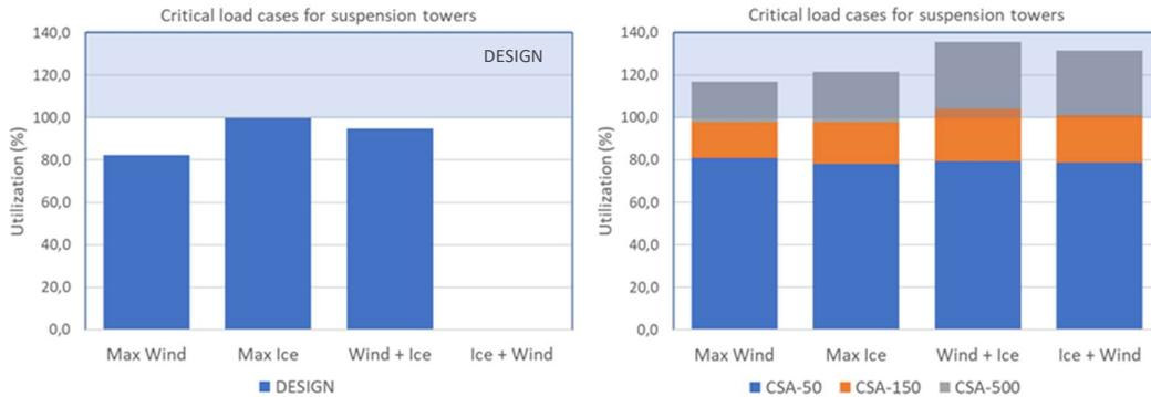
**FIGURE 24** Highest utilization in suspension tower for each load case.
