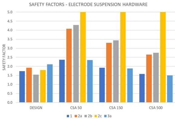
FIGURE 37 Safety factors for electrode suspension hardware per loading type for each zone.
