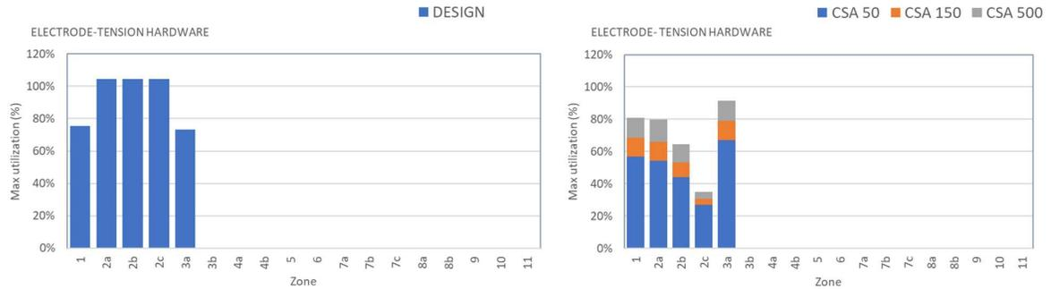
FIGURE 38 Electrode conductor tension hardware. Maximum utilization per zone of DESIGN<sup>21</sup> and CSA- loads is presented.
