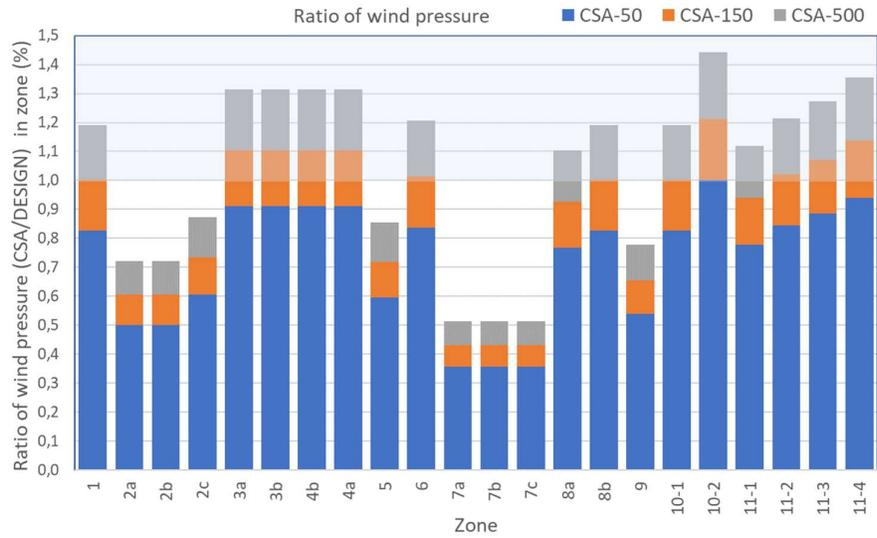
**FIGURE 18** Ratio of wind pressure according to CSA (50, 150 or 500) against DESIGN wind pressure.
