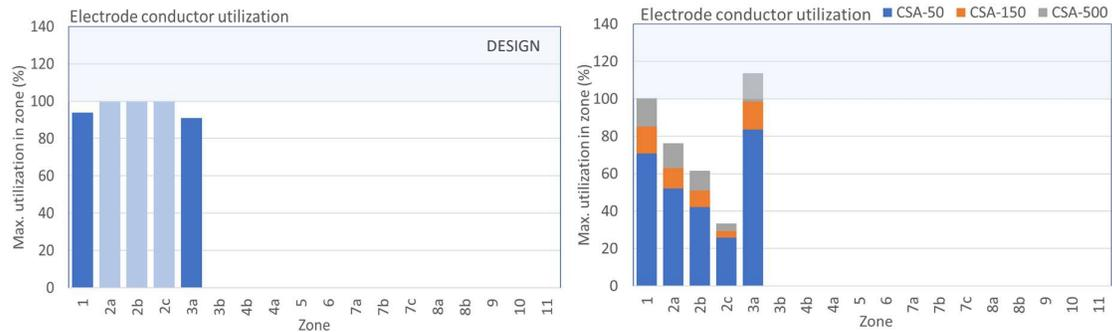
**FIGURE 31** Electrode Conductor, highest utilization in each loading zone. Utilization in DESIGN loading<sup>21</sup> is to the left and CSA loading to the right.
