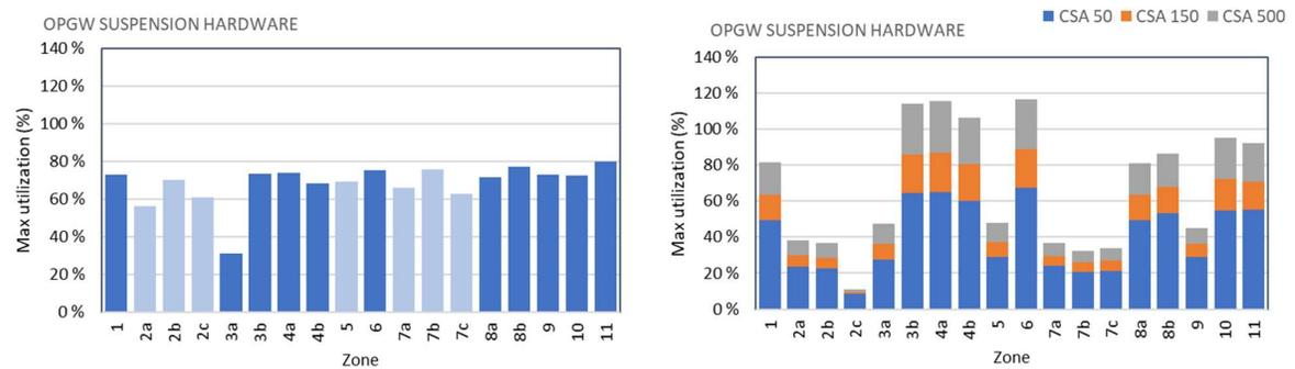
FIGURE 40 OPGW suspension hardware. Maximum utilization per zone of DESIGN<sup>21</sup> and CSA- loads is presented.
