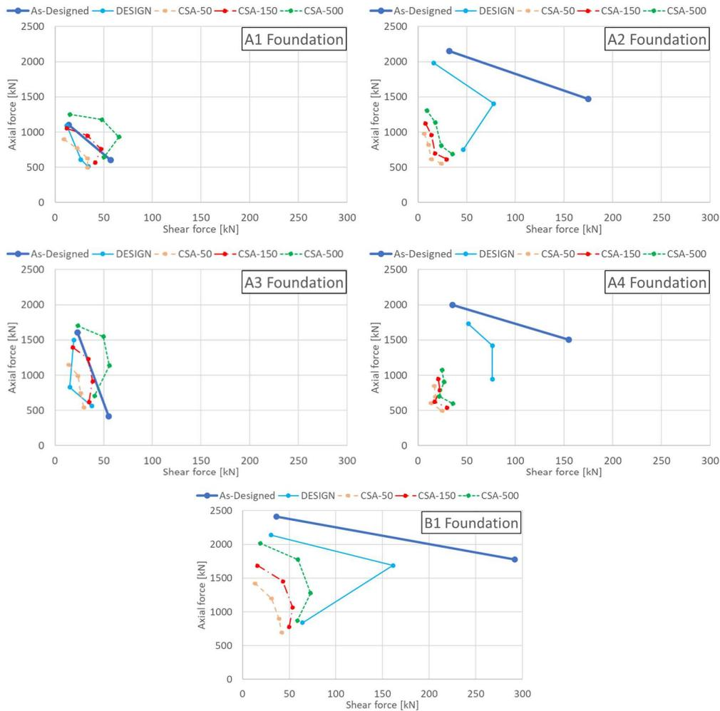
**FIGURE 27** Maximum foundation forces in guyed suspension towers. Each figure shows: two load combinations used in the design (“As-Designed”) and maximum combinations of the load cases “Max. ice”, “Ice&wind”, “Wind&Ice” and “Max. Wind” for each of the load groups: DESIGN, CSA-50, CSA-150 and CSA-500. All values are presented without strength factor.
