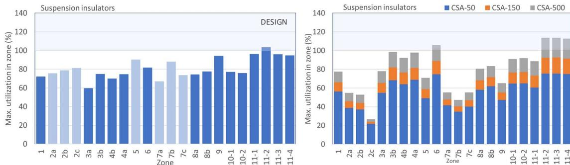
**FIGURE 33** Suspension insulators, highest utilization in each loading zone. Utilization in DESIGN loading<sup>21</sup> is to the left and CSA loading to the right.
